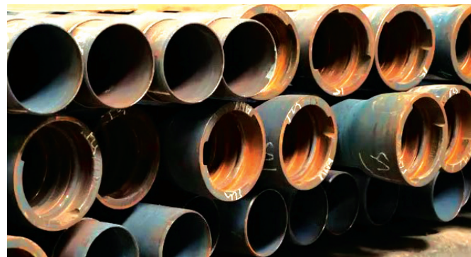
Cast Iron Pipes
